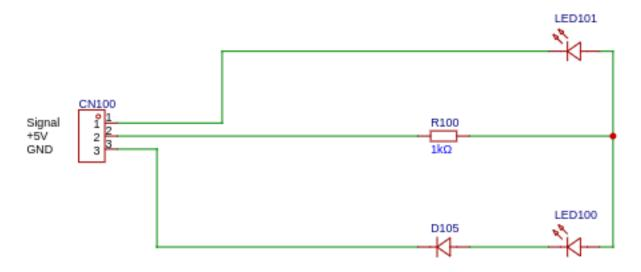
The diagram above is one way to wire up the leds for connection to the RT\_Pulse\_8\_Servo decoder. LED2 will be the active led when a throw command is issued for the relevant output. This method provides an indication if in the close or thrown position.
