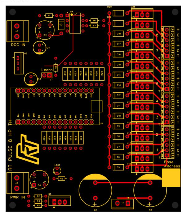
As with most PCB construction start with soldering in the lowest profile items first, eg resistors, diodes, leds, etc.
